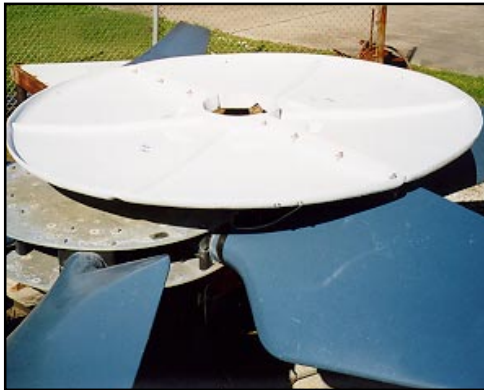
Typical Seal Disc Prior to Installation Fig. 13
